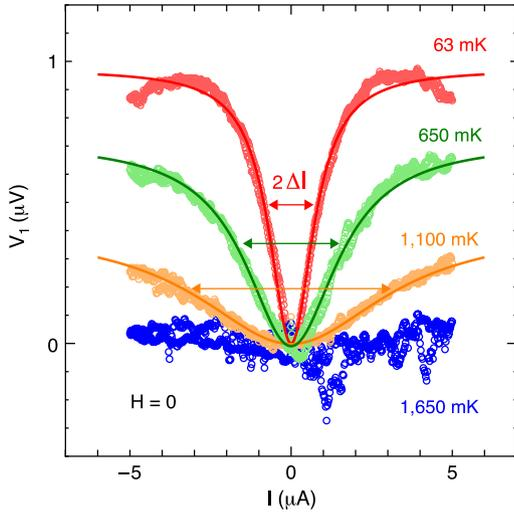
**Fig. 3.** The anomalous nonlinear voltage (ANV) which is described by the voltage  $V_1$  is extracted from  $I$ - $V$  characteristics in Fig. 2, where the lines are Lorentzian fitting curves. The half-widths  $\Delta I$  of the fitting curves are represented by two-headed arrows. We eliminated the offset voltage of  $0.13 \mu\text{V}$  in order to discuss the ANV.
